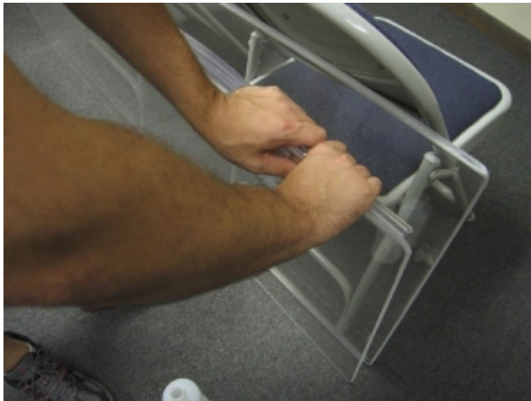
3. Snap hinge into groove on one panel by pressing straight down
