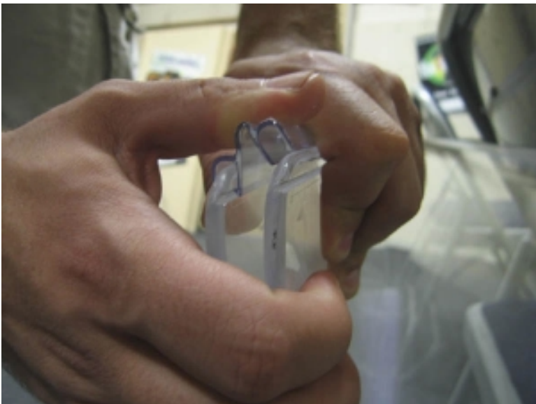
5. Bend hinge over onto adjoining panel and snap into groove. Attach completely to entire length of adjoining panel.
