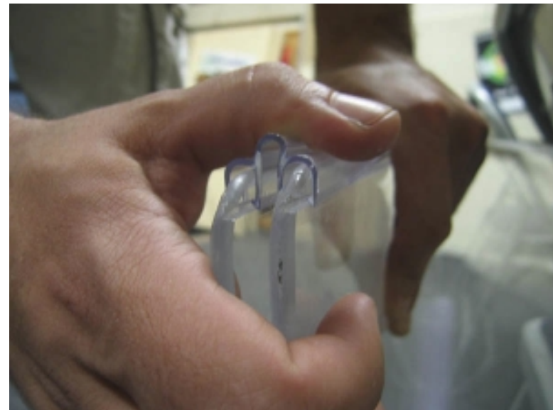
5. Bend hinge over onto adjoining panel and snap into groove. Attach completely to entire length of adjoining panel.
